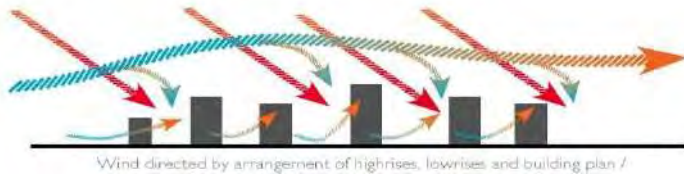
Wind directed by arrangement of highrises, lowrises and building plan /
