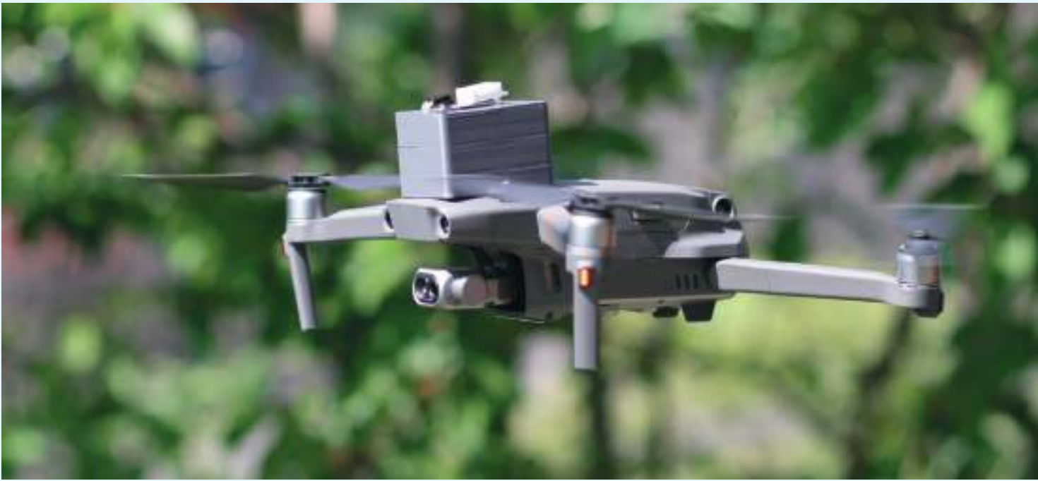
Use of an UAV for Remote Sensing Application: DJI Mavic 2 Enterprise with Thermal Camera (Fig. 17)
