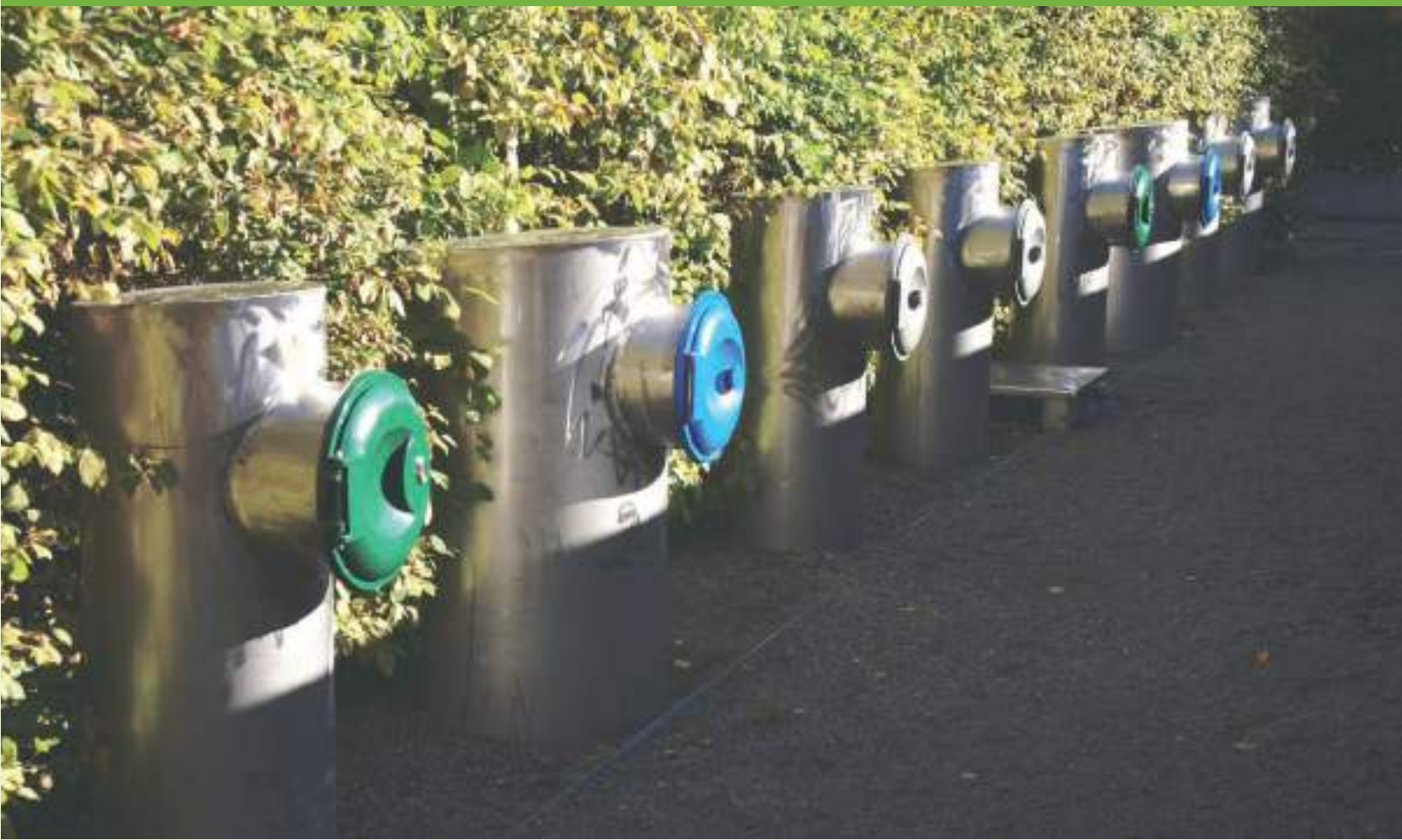
Waste collection station: Above ground, collection points for paper, metal, glass and plastic waste are located on each building block. Non-flammable components are collected and fed into the recycling cycle. Hazardous waste such as paints or batteries are collected centrally for appropriate disposal. (fig. 8)
