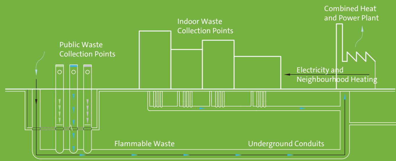
Waste collection with underground vacuum system (fig. 7)
