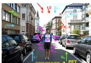
Schematic overview of both heat fluxes within an urban street canyon and human heat fluxes leading to the quantification of the human perception of heat by PET (M: metabolic rate, Q_{net} : latent heat flux, Q^* : net radiation, Q_{sw} : heat flux due to solar radiation, Q_{lw} : heat flux due to longwave radiation, Q_{res} : heat flux due to respiration, Q_{sk} : heat flux due to skin, Q_{cl} : heat flux due to clothing).
