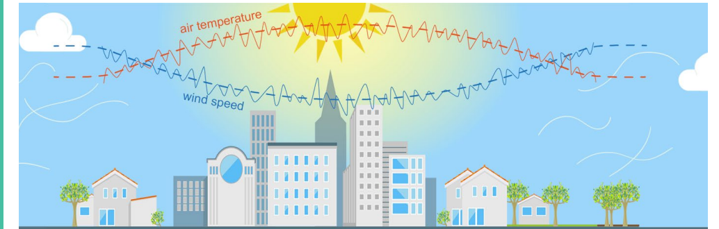
Figure 20. In urban areas, reduced wind velocity is closely linked to high building density and the absence of planned ventilation corridors. This limited airflow traps heat, intensifying the urban heat island effect and exacerbating temperature increases, especially during summer and heatwaves.
