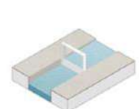
sluice gate as movable closure tidal gate/ navigation lock
