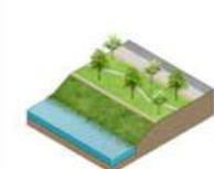
ground raising with green embankment
