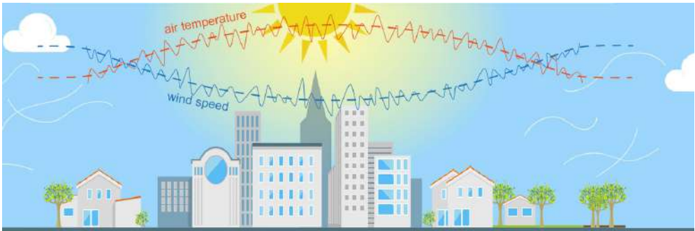
Figure 20. In urban areas, reduced wind velocity is closely linked to high building density and the absence of planned ventilation corridors. This limited airflow traps heat, intensifying the urban heat island effect and exacerbating temperature increases, especially during summer and heatwaves.
